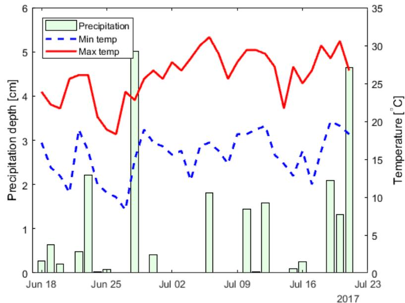
Figure 4.2: Precipitation and temperature records for Madison, WI June 18 to July 21, 2017 indicate this was a relatively wet period of the summer, but also relatively mild as the maximum temperature was 31°C.
