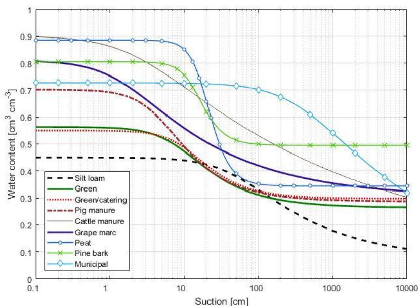
Figure 4.6: Graphical representation of the van Genuchten fitted soil water characteristic curves for the underlying silt loam soil and the assessed composts. While there was a wide range of saturated and residual water contents, most composts began losing water between 5 cm and 10 cm of suction head.
