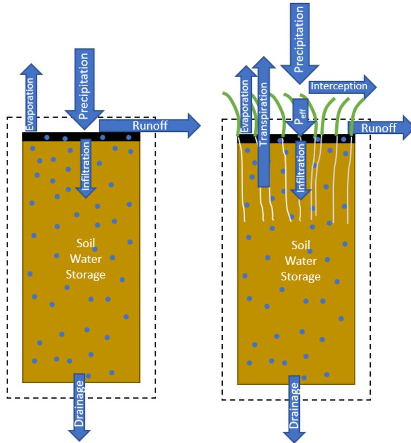
Figure 4.1: Conceptual diagram of an unvegetated compost blanket (left) and vegetated compost blanket (right) indicating different fluxes entering and exiting the control boundary
